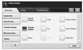
For example, if you want to change the default setting of the brightness & darkness for a copy job, press **Copy** > **Darkness** and adjust the brightness & darkness.
